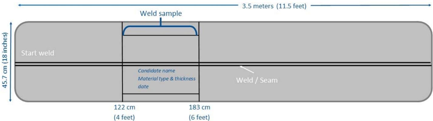
Cut the two-foot submission coupon starting at the 122 cm (4 feet) mark.
