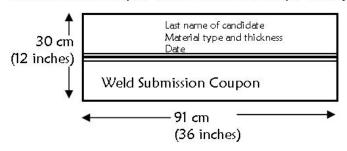
Cut the submission coupon starting at the 122 cm (4 foot) mark. This allows for temperature drop and recovery period on fusion welds.
