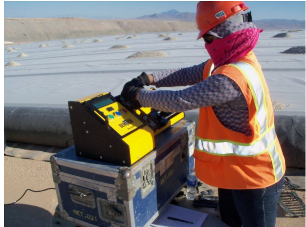
Demtech photo testing seams on tensiometer
