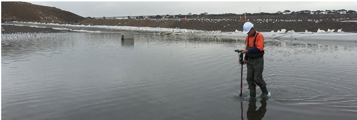
Layfield Canada technician dipole testing process water mining pond in Northern Saskatchewan
